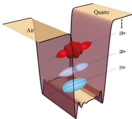
**Figure 1:** A metal quantum well structure is formed based on an ultrathin gold film sandwiched between the quartz substrate and air on top. The first three lowest energy levels and their corresponding wave functions are also sketched. The shape deformation of the well bottom indicates the impact of electron distribution.
