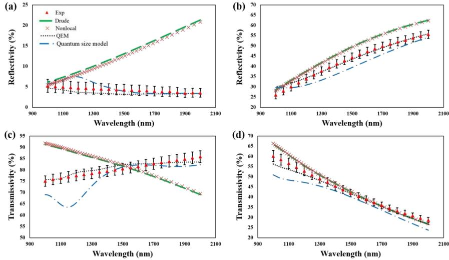
**Figure 4:** Comparison between reflection (top) and transmission (bottom) for 2.5 nm (a and c) and 7 nm (b and d) gold films for which the refractive index  $n$  and  $k$  are from the Drude model, nonlocal model, quantum size model, and quantum electrostatic model. The corresponding experimental results are marked by red triangles.
