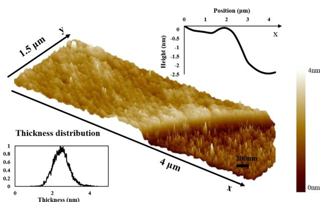
**Figure 2:** Atomic-force microscopy image of one of the 2.5 nm thin gold films, showing the film edge on the substrate. The upper inset shows the averaged height on both sides across the edge (the mean thickness), indicating the mean thickness of the film is about 2.5 nm. The lower inset shows the surface roughness is around 0.5 nm.
