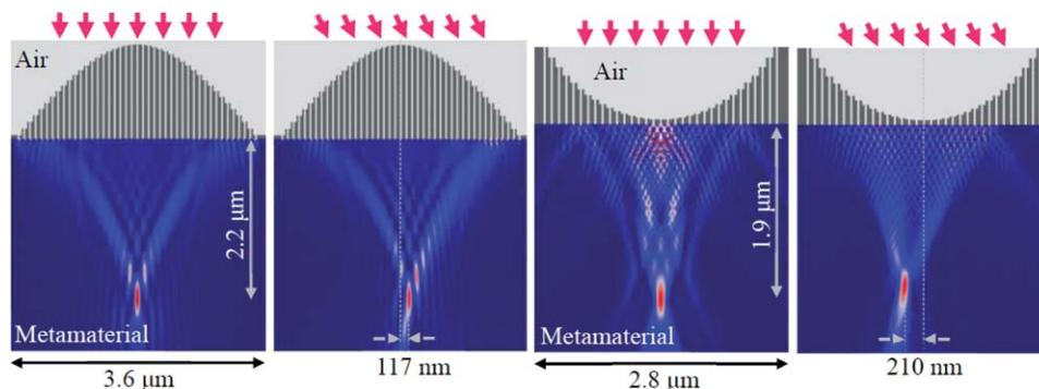
**Fig. 5** Simulations of an elliptic metalens with a height tuning PWC, illuminated by (a) a normal and (b) a tilted plane wave, respectively, and simulations of a hyperbolic metalens with a height tuning PWC, illuminated by (c) a normal and (d) a tilted plane wave, respectively.
