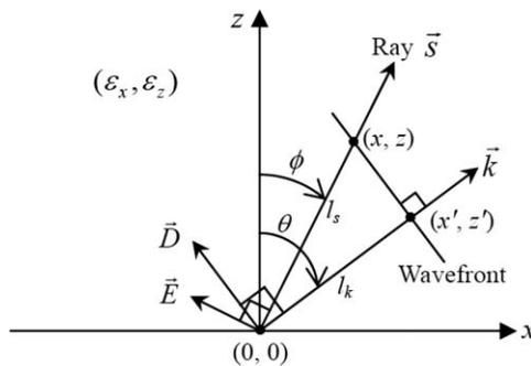
**Fig. 3** Group velocity (ray direction) and phase velocity (wavevector  $\vec{k}$  direction) of a ray in a uniaxial anisotropic medium with permittivities  $(\epsilon_x, \epsilon_z)$ .
