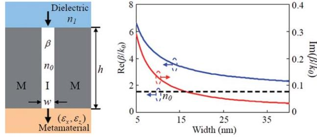
**Fig. 2** (a) Schematic of a MIM waveguide above a metamaterial. (b) Dependence of the modal index of a nanoscale MIM waveguide on the width  $w$  of the insulator layer. The upper curve represents the real part and the lower curve represents the imaginary part. Data obtained using infinitely thick silver and a dielectric with a refractive index  $n_0 = 1.5$ . The dashed line represents the propagation constant of a plane wave in the core dielectric material  $n_0$ .
