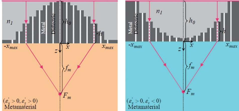
**Fig. 4** Schematics of (a) an elliptic metalens and (b) a hyperbolic metalens with a height tuning PWC.
