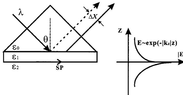
FIG. 1. Kretschmann–Raether ATR configuration, with the metal thin film ( $\epsilon_1$ ) coating. The solid reflective beam shows a positive optical beam shift compared to the geometrical reflection ray (the dashed line). The insets show the exponential dependence of the electrical field along the metal–air interface.
